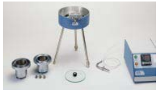
Temperature cups with threaded base that attaches to a water bath stand and "Electemp" temperature control unit.
