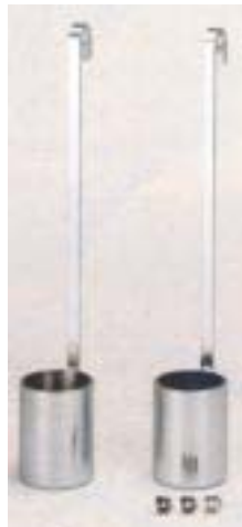
Cups with handles. Models DIN 53211 No. 4 and Ford ASTM D-1200.
