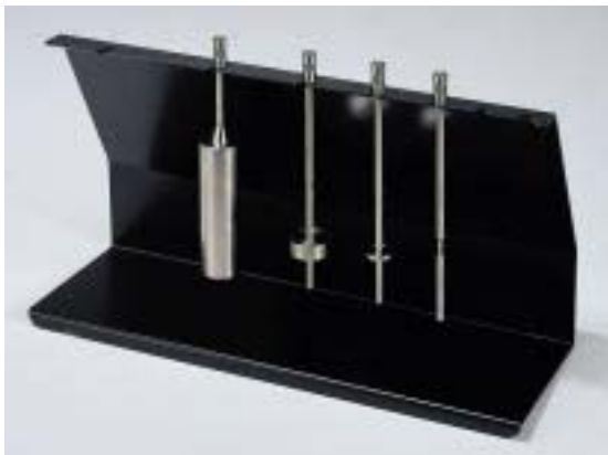
Rack support for spindle standards L1, L2, L3 and L4 for the ST-DIGIT L.
