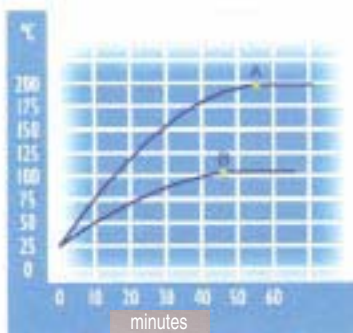
Graph of temperature and time for the Tectron-Digitem 100 and 200, units with capacity of 20 litres. Tests completed with Silicon oil:
